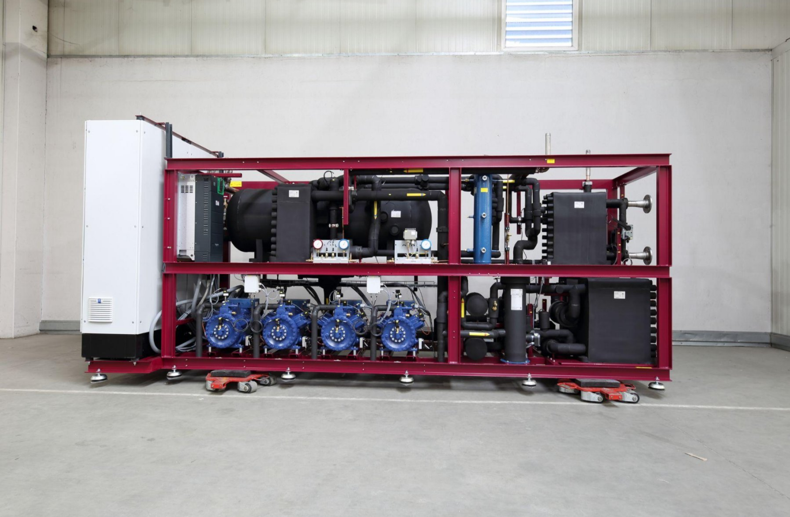
The CO 2 chiller with integrated heat recovery TEKO built for an Italian winemaker. Photo credit: TEKO
