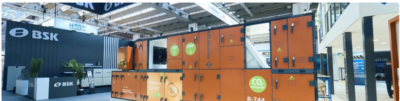
The Menerga CO 2 mpass, an air-handling unit with an integrated CO 2 heat pump, on display at ISH 2025. Photo credit: Systemair
